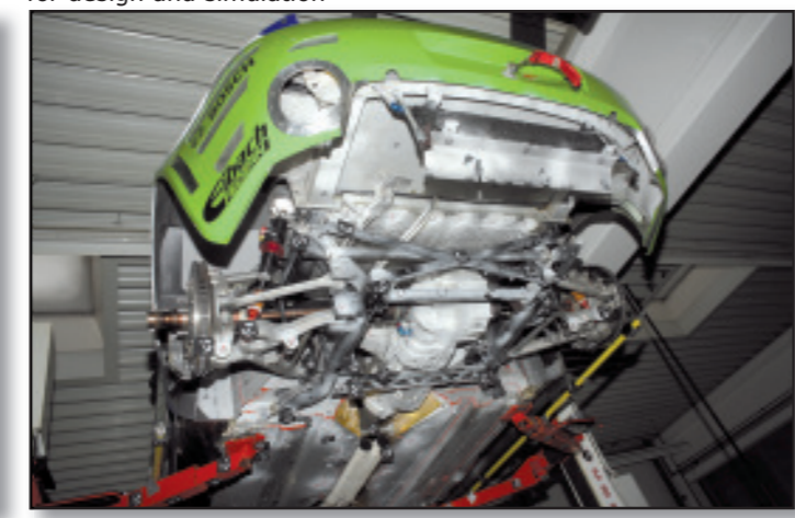
Rapid chassis measurement using photogrammetry for design and simulation
